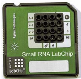
Example of a microfluidic electrophoresis chip For the Agilent 2100 Bioanalyzer (actual size)
