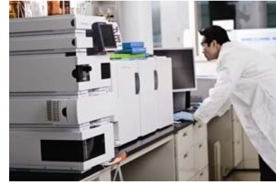
Agilent 1200 Series Rapid Resolution Liquid Chromatography System coupled to an Agilent Accurate Mass Quadrupole Time-of-Flight Mass Spectrometer
